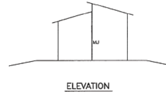
Figure 7.11: Geometrical change in wall height, i.e., single storey to two storey walls.
